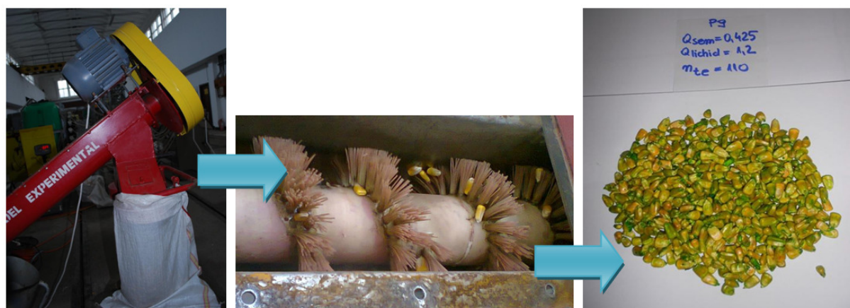
Fig. 3. Seed sample taken at the exit of the helical conveyor
